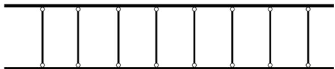
**Figure 3. Beam differentiation using the shear analogy method: Beam A at the top with bending stiffness  $(EI)_A = B_A$ , and shear stiffness  $(GA)_A = S_A \sim \infty$ ; Web members in the middle with infinite axial rigidity; and Beam B at the bottom with bending stiffness  $(EI)_B = B_B$ , and shear stiffness  $(GA)_B = S_B$ . [5]**
