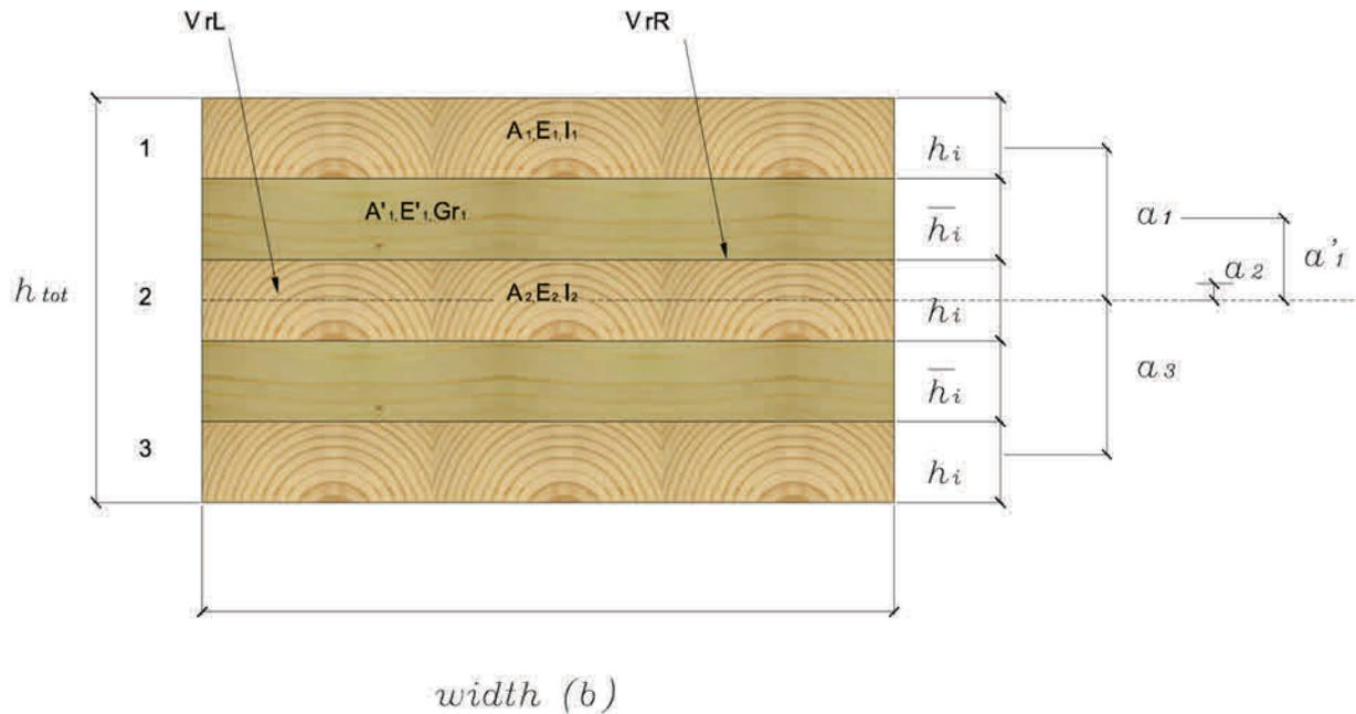
Figure 2. Cross-section of CLT panel with five layers
