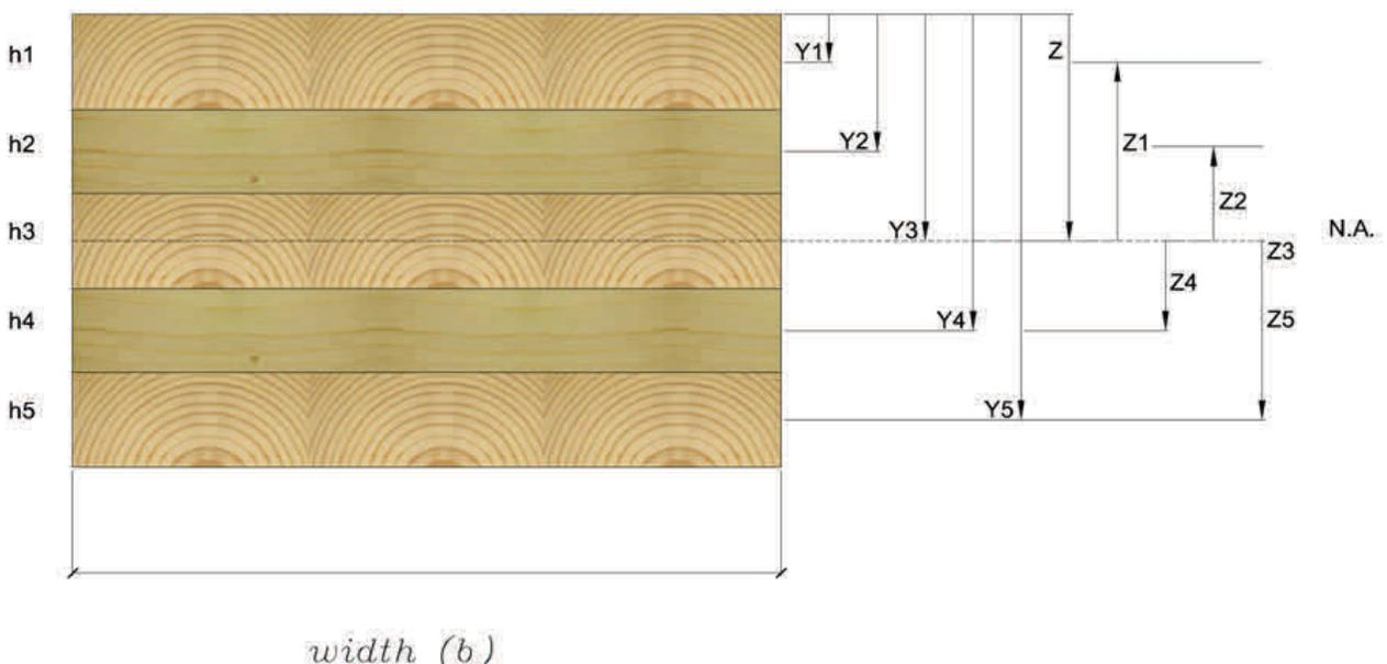
Figure 4. Cross section designations in a five-layer CLT panel
