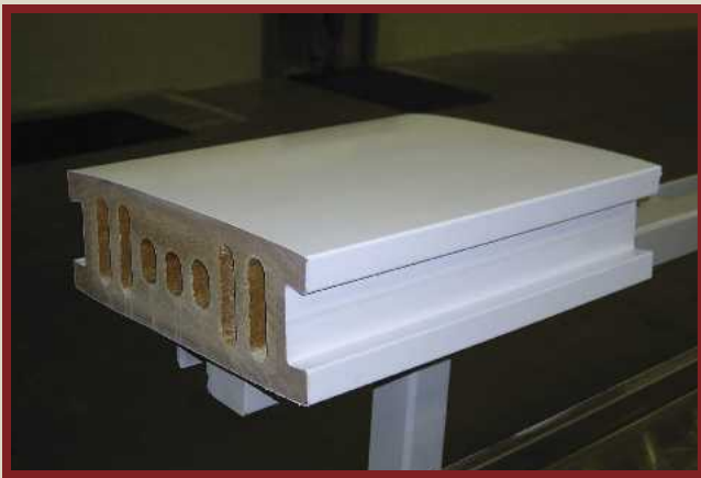
Figure 1c. — Prototype 4 by 12-inch capped industrial WPC deckboard. This deckboard, and the deckboard on the cover of this issue, were extruded at Strandex Corporation’s research and development laboratory in Madison, Wisconsin. These industrial deckboards were developed under sponsored research from the Office for Naval Research (ONR) by Washington State University and Strandex Corporation and are being commercially produced by a Strandex licensee and distributed by McFarland Cascade Corporation. These products are being deployed in demonstration projects such as a trail bridge near Missoula, Montana (in cooperation with the USDA Forest Service Wood-In-Transportation Program) and a new pier at the U.S. Naval Academy in Annapolis, Maryland.
